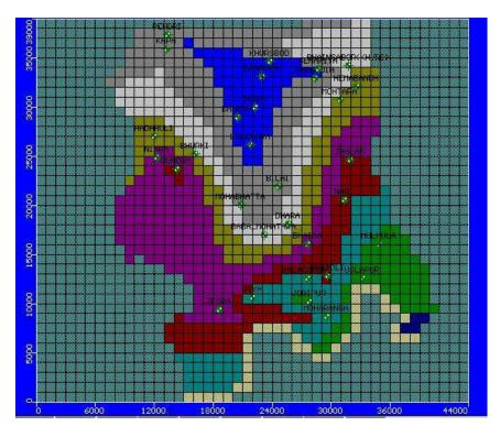
Fig.45. Initial Heads of the First Layer as Simulated from the Observed field data
