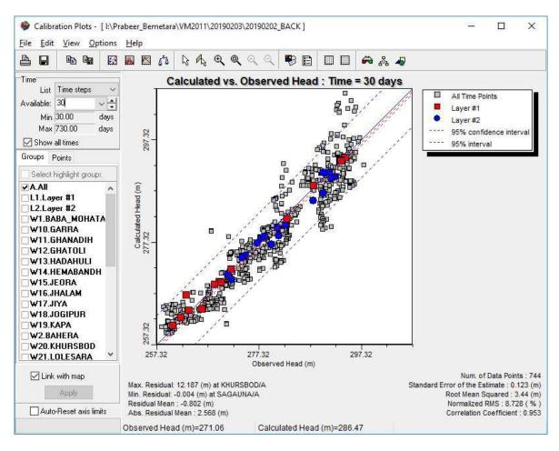
Fig.48. Calibration Plot of Observed head versus Computed head
