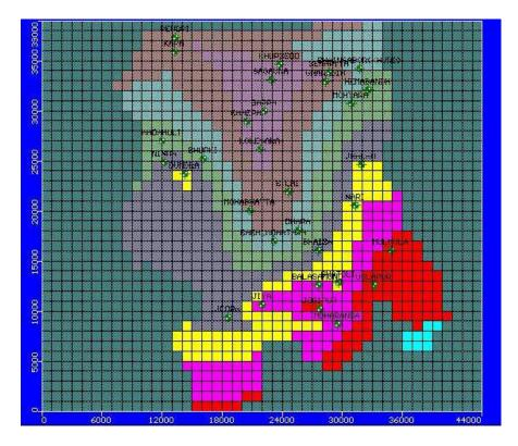
Fig. 46. Initial Heads of the Second Layer as Simulated from the Observed field data.
